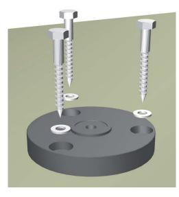
The central plate for the rotor must be secured with  $3x \Phi 12$  screw plugs, washers and 10x80mm hexagon-head bolts.
